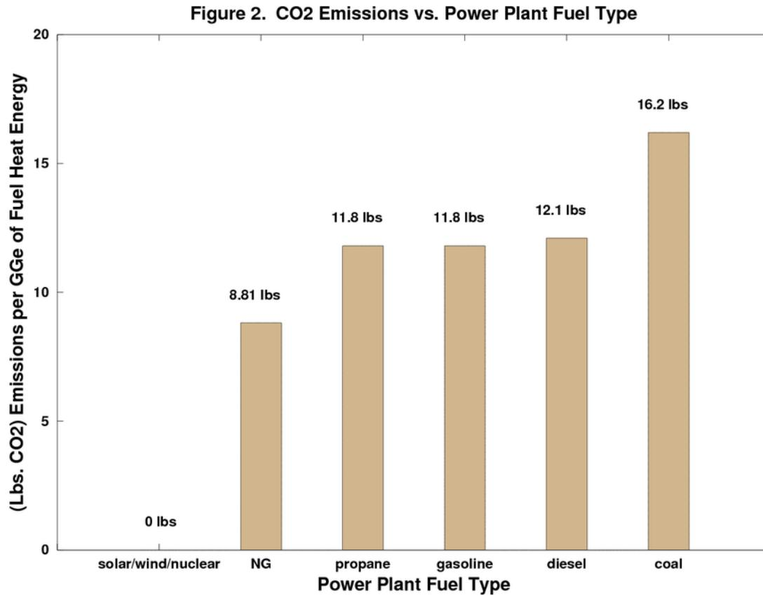
Figure 1 and 2 information were used to produce Figure 3 which shows the average number of pounds of CO<sub>2</sub> emitted per power plant fuel type to deliver one GGe unit of electricity over the present day NJ electric grid for charging an electric vehicle battery.
